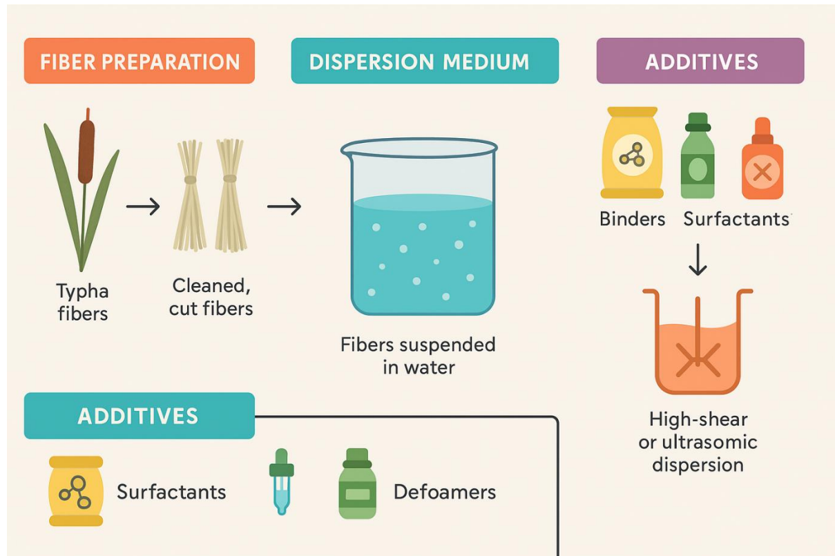
Figure 3: Wet-laid non-oven production using typha fibres
