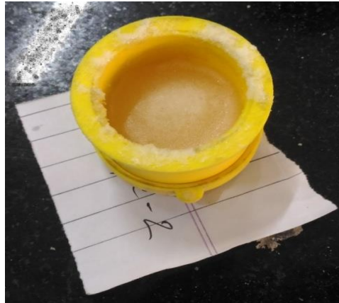
Fig 6: Cold Setting using Hardener in the Moulds
