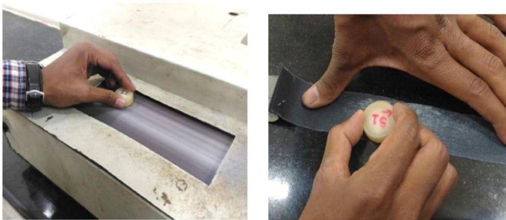
Fig 7: Workpiece Grinded in the Belt Grinder & Polishing with Silicon Carbide Paper
