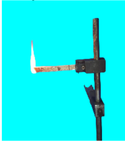
Fig 5 Burning test of natural fibre
