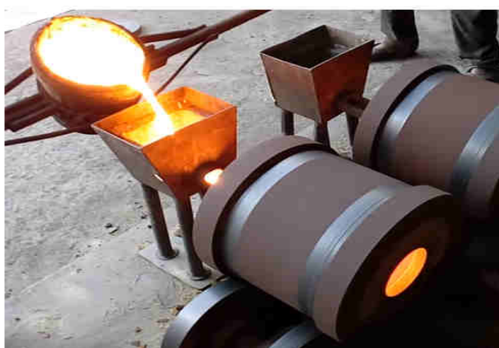
Fig 1 Horizontal Centrifugal Machine
