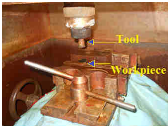
Fig. 2 Mild steel workpiece and tool
