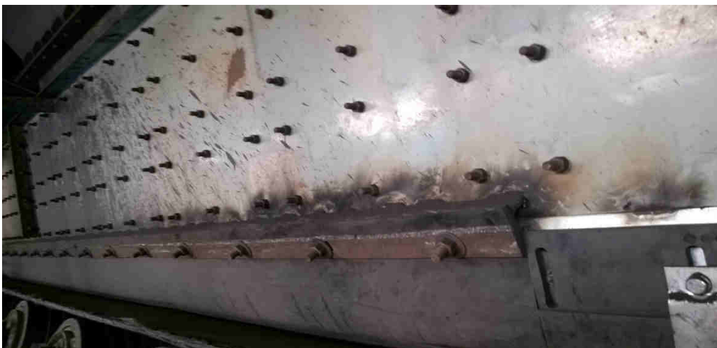
Fig 2. Rubber pad after modification
