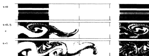
Fig. 3 Results for a baffled channel with no oscillatory component in the flow at Re = 300 .
