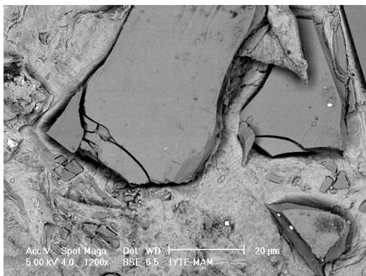
**Figure 4.** SEM images of the failed 0/10/20 sample 0/10 interface tested at 90 psi showing fractured SiC particles.
