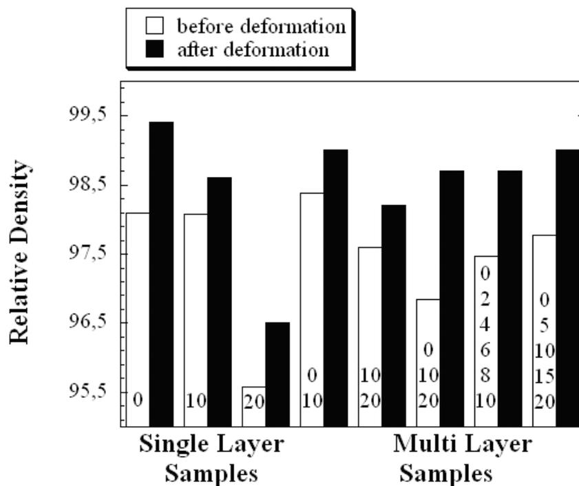
**Figure 3.** Relative densities of single and multiple layers
