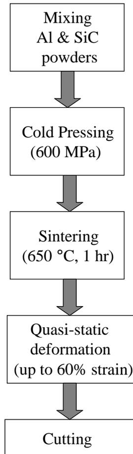
**Figure 2:** Schematics of sample preparation
