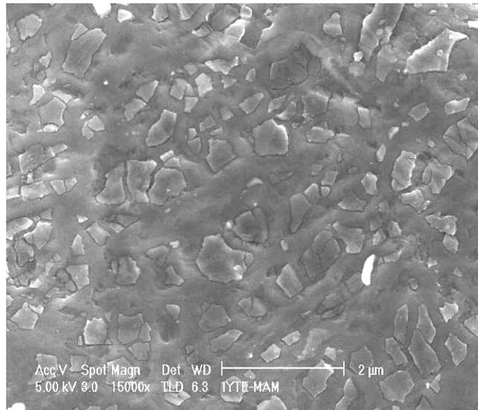
**Figure 5** SEM images of the failed 0/10/20 sample 0/10 interface tested at 90 psi showing oxide plates.
