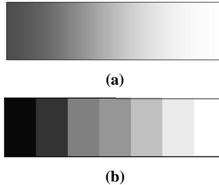
**Figure 1** Gradient architecture of FGMs; (a) continuously graded and (b) discretely layered FGMs.
