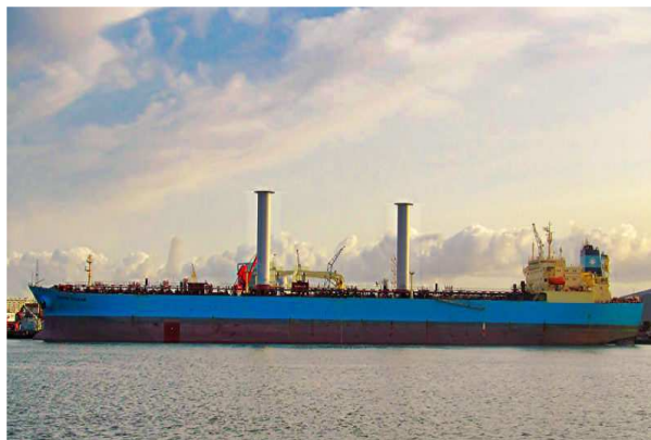
Fig 3 ROTOR Sails installed on Maersk Pelican (8.2% fuel savings were accounted)
