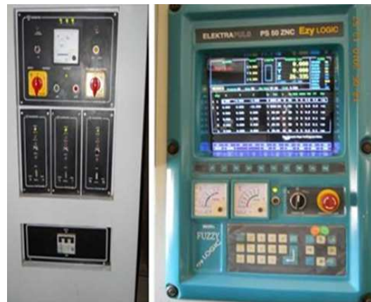
Fig. 3 Control unit of EDM machine [16]
