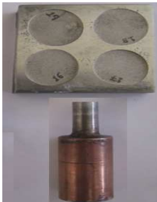
Fig. 4 Machined workpiece and Tool
